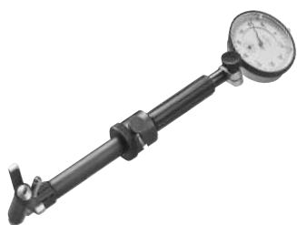
Model 264-010 with fixed contact point turned in. Contact will rotate 180° to measuring position once gage enters part.
