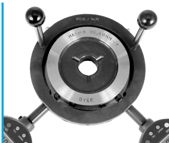
283 Special OD gage position on cylinder master.
