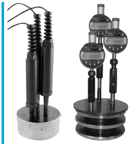
3 Ø's, Taper, out-of-round, TIR
