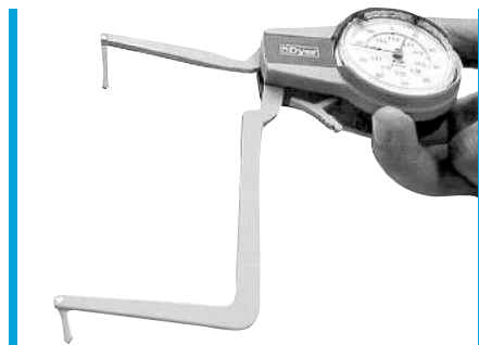
104 Series special Right angle contacts to measure recessed grooves around a hub.
