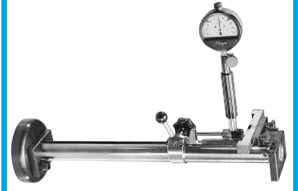
222 Series short handle gage with adjustable setting master.
