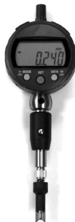
438 Series keyway gage with 209-020 retractable handle and 900-105 electronic indicator
