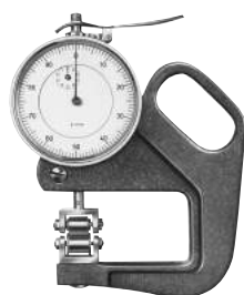
305-555 Thickness Gage, Roller Contacts Range: 0-0.2" Grad: 0.001" Width of roller = 0.34" Measuring force = 120 gm.
