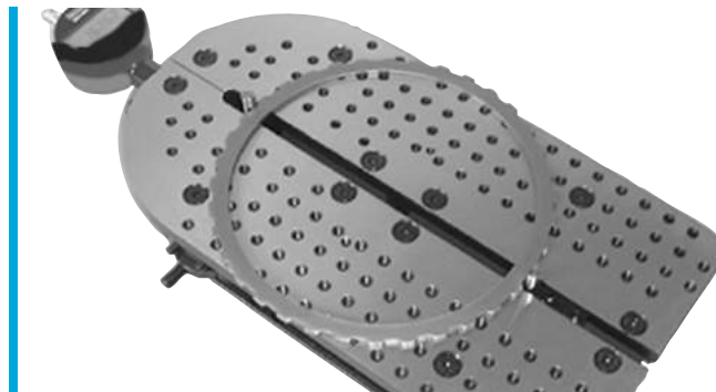
747 Series Measure external splines at 2 positions
