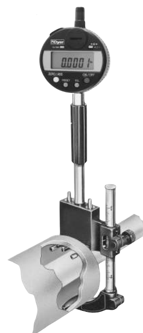
The gage will set flat against the part allowing the gaging to be electronic and non-tipping with no operator influence.
