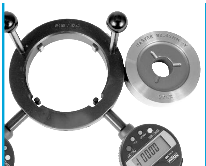
283 Special OD gage to measure splined part.
